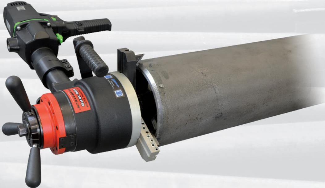
PRO-10 PB is a heavy duty pipe Beveler designed for portable use in pipe machining operations. Self-centering expandable mandrels provide quick and proper alignment to a pipe or a tube prior to machining operations.
