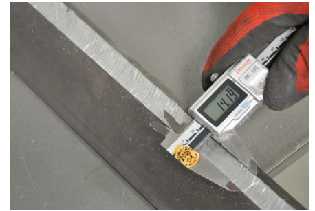
Maximum bevel width up to 14 mm
